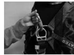
After 3 point attachment, ensure carabiner is loaded correctly.
