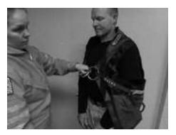
A.R.V. is secured in place via gathering the three attachment rings (L/R sternal and lower) and securing with the supplied steel auto-locking carabiner.
