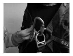
**Carabiner is used for direct** attachment to hoist hook, short haul line assembly, or other rescue system.
